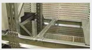
Fixing over the front and rear beams these bars support undersized or damaged pallets.
