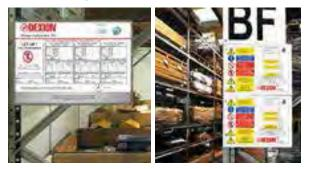
Load signs indicating load capacities must be fitted on all racking and shelving. They must be clearly visible for all users.
