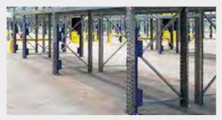
A load bearing section is added to the initial 1000mm of an aisle facing upright. A removable piece of upright is then fitted to the front, this is not load bearing and can easily be replaced if damaged, without the need to unload the complete bay.
