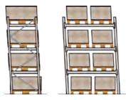
**INCLINATION** Maximum inclinations for both empty and fully loaded racks should not be exceeded.
