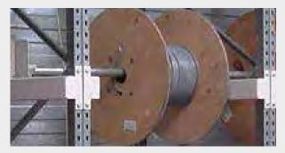
For storage of large cable reels or carpet rolls. A supporting rod, with high weight capacity, can easily be taken in and out of position.
