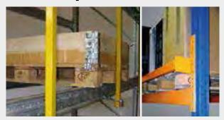
A useful safety feature which prevents pallets from falling from the back of the rack.
