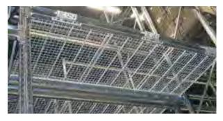
Mesh Shelves are used above tunnel bays to protect against goods falling down.
