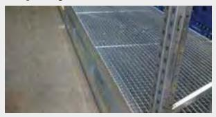
If liquids might leak, then drip trays may be placed on the floor (or per level). The drip trays are galvanized. Various sizes are available.
