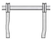
**DEFORMATION** Even slightly bent beams and uprights can be a sign of potential danger. Beams and uprights must always be replaced.
