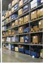
The new central warehouse of Volkswagen contains 100,000 spare parts across the VW range. Pallet racking with 12,300 pallet places guaranteed full accessibility and safe storage of all items.
